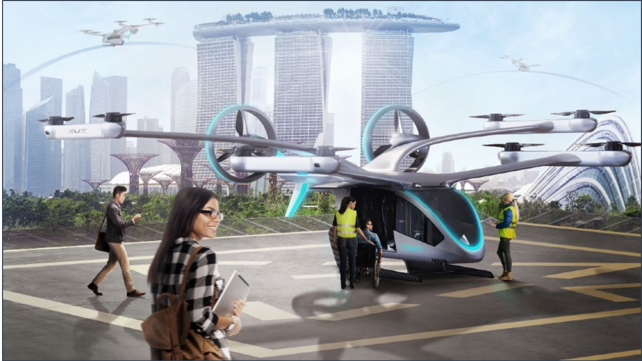
Figure 16 - As eVTOL aircraft emerge and become certified for operation above cities and regions, on-demand air taxi concepts will take hold. eVTOL aircraft will need landing pads called “vertiports” sited at convenient locations such as airports, hospitals, downtown, major trucking and distribution companies, and headquarters of large corporations.
