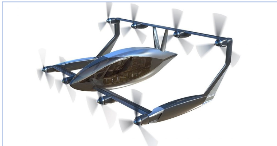
Figure 9 - Due for commercial release in 2023, Vertiiia could be the world's first eVTOL aircraft designed exclusively for aeromedical transport. Its small dimensions allow for close-in operations at the site of patient transport.
