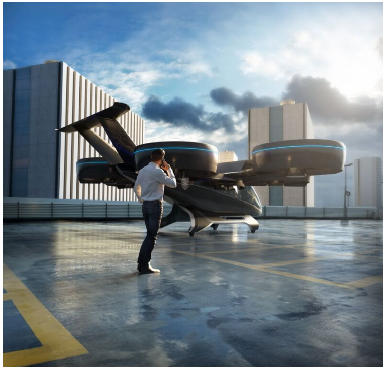
Figure 2 - The Bell NEXUS Six Rotor, Five Passenger Hybrid Electric VTOL Aircraft Can Cruise at 200 Miles per Hour.
