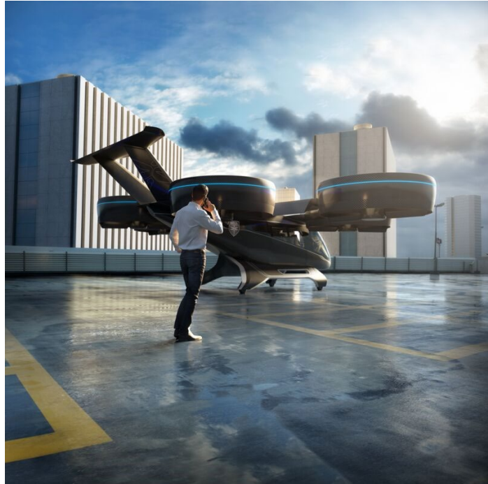
Figure 2 – The Bell NEXUS Six Rotor, Five Passenger Electric Hybrid VTOL Aircraft Can Cruise at 200 Miles per Hour.
