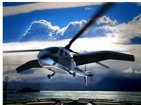
Figure 6: Piasecki Aircraft PA890 electric VTOL designed for long range medevac uses.
